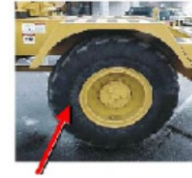
A cut in the sidewall of a crane tire is considered a major deficiency (load bearing/load controlling) if the crane is certified for on-rubber lifts.
