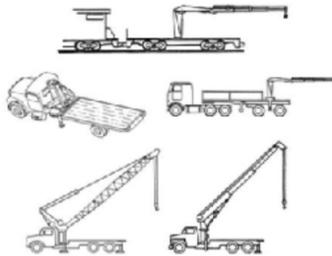
**Booms and Mounts:** Category 4 cranes have different types of boom configurations such as: telescoping, non-telescoping, and articulating. They may be mounted on flatbed trucks, trailers, stake beds, rail cars, barges and pontoons, or may be stationary mounted on piers, wharves, and docks.
