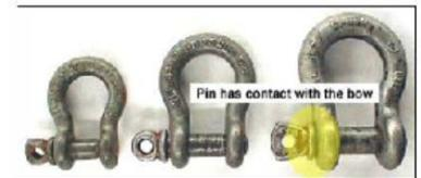
When side loading screw pin or bolt type shackles:
