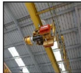
Trolley Mounted Overhead Hoists
