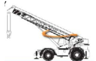
4. Select the best answer to fill in the blank. When moving a truck, cruiser, or crawler crane to and from job sites, always secure the \_\_\_\_\_ to the carrier frame.
