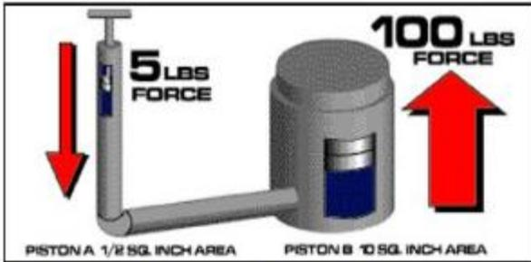
The difference in the areas of the two pistons determines the multiplication of force.
