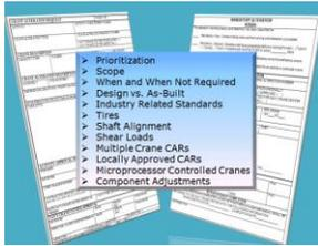
What is in appendix O? Appendix O discusses the prioritization and scoping of alteration requests, when alteration requests should and should not be used, design and as-built considerations, and industry standards related to the certification of weight handling equipment. See the list on the screen for additional topics contained in appendix O.
