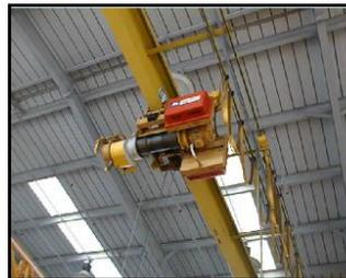
Trolley Mounted Overhead Hoist
