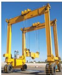
A rubber tire gantry crane may be single beamed or double beamed. Often it resembles a mobile bridge crane with its hoist mounted on a bridge which spans two beams. As shown in the illustration, it may be configured with two hoists mounted on opposing beams which utilize a spreader bar or similar mechanism to lift loads. The gantry style legs allow the crane to hover over loads, improving stability. The wheels and rubber tires may be motorized or non-motorized.
