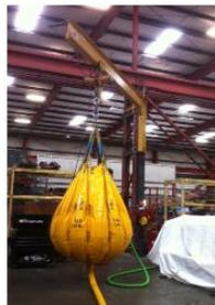
*Jib crane load test.*
