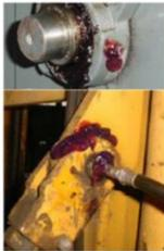
The quantity of grease is important. Remember, too much grease is as detrimental as insufficient grease.
