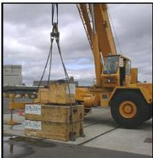
The procedures for load testing are covered in a separate module, which will be presented for those who are or will be designated as test directors. In general: Load tests are conducted by a load test director. As an inspector, you will be required to sign the Certification of Load Test and Condition Inspection, verifying that you have conducted inspections of the crane.
