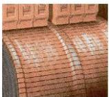
Grooving is noted by a distinct loss of material in the brush path. This condition can be caused by improper brush-hardness or brush tension, to current balance. This can be corrected by machining the commutator to restore an even surface and replacing the brushes with the correct brushes adjusted to match the current ratio.
