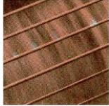
A heavy dark film over the entire surface can be cleaned with folded canvas applied to the running commutator.
