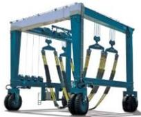
A mobile boat hoist consists of a steel structure of rectangular box sections, supported by four sets of wheels capable of straddling and carrying boats.
