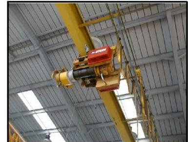
Trolley Mounted Overhead Hoist
