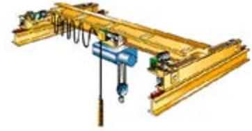
Operators should always check for trolley and bridge drift before operating the crane.
