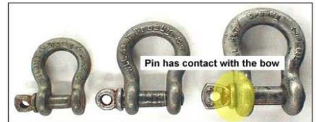
When side loading screw pin or bolt type shackles:
