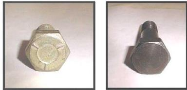
manufacture to identify their product. Bolts without these identifying marks should be immediately suspect. Lists are available showing the head markings of fasteners which have proved to be counterfeit. For information on the Fastener Quality Act, registered head markings or a list of counterfeit head markings, visit the web sites shown.
