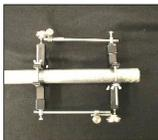
to determine the distance between the brackets and how long the rods will have to be for the indicators to make contact with their opposing bracket. Next, detach the set-up from the machine shafts. Using the dimensions established from the previous step, re-attach to a piece of thin-walled tube or light pipe so that the indicator sag may be measured
