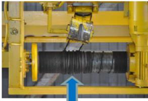
IMPROPER SPOOLING / DRUM MIS-SPOOL
