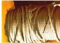
Mis-spools cause: flattening, crushing, abrading, distorting or kinking of the wire rope
