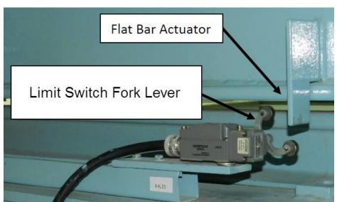
Similarly, at a Navy activity, a limit switch is used to slow the crane as it approaches the end stops. In this case, a rotary limit switch is located on the crane end truck, as shown below, and the actuator is mounted on the crane runway.
