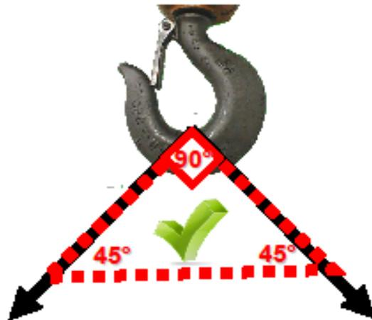
Improper hook use and attachment of rigging gear **may result in damage to equipment and/or personnel injury or death.**
