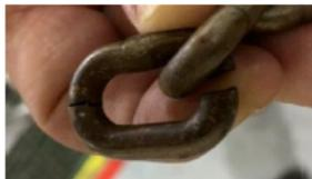
**FAILURE:** Chain was used over a chemical dip tank and chain-link failed during use.
