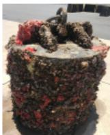
**FAILURE:** Chain was submerged in a marine environment and chain-link failed during use.
