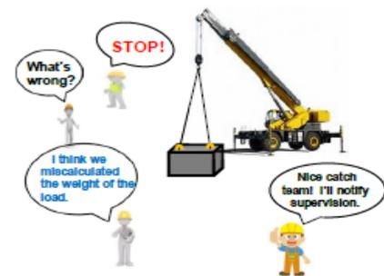
Be alert! Always know the weight of the load, capacity of the rigging gear's weakest link, and capacity of the crane as configured!
