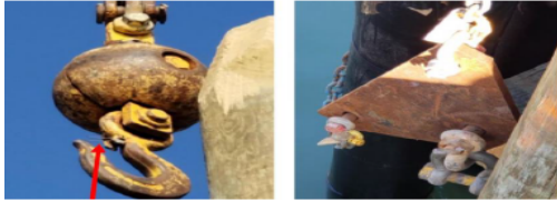
Broken Safety Latch → 120 pound spreader fell onto 2 workers.
