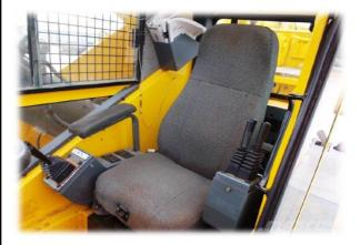
Operational Safety Devices – In addition to the typical Load Moment Indicator or Rated Capacity Limiter mobile cranes are often equipped with other functional interlock devices such as operators seat or push button "deadman" switches or moveable armrest console that disable all functions when tilted back.
